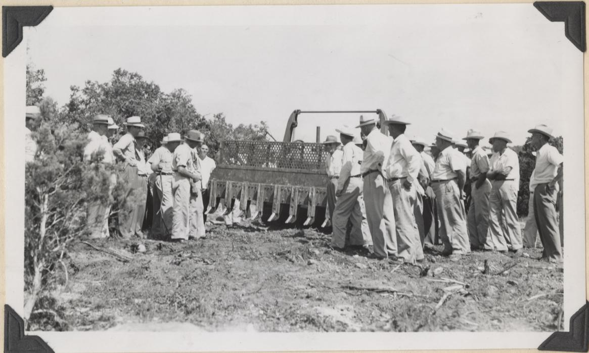
Eradicating brush on cut-over and burned-over cedar land with a medium sized crawler tractor, equipped with a specially designed grubber was demonstrated to Travis County ranchers on a field trip in September. The equipment was designed and demonstrated by Basdall Gardner on his own ranch near Leander in Travis County.
